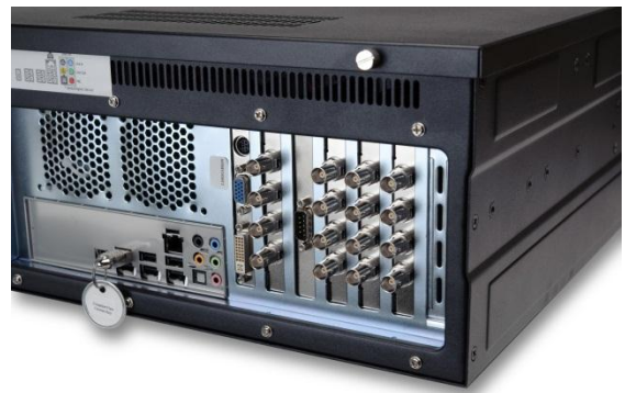
Server with video capture cards installed
